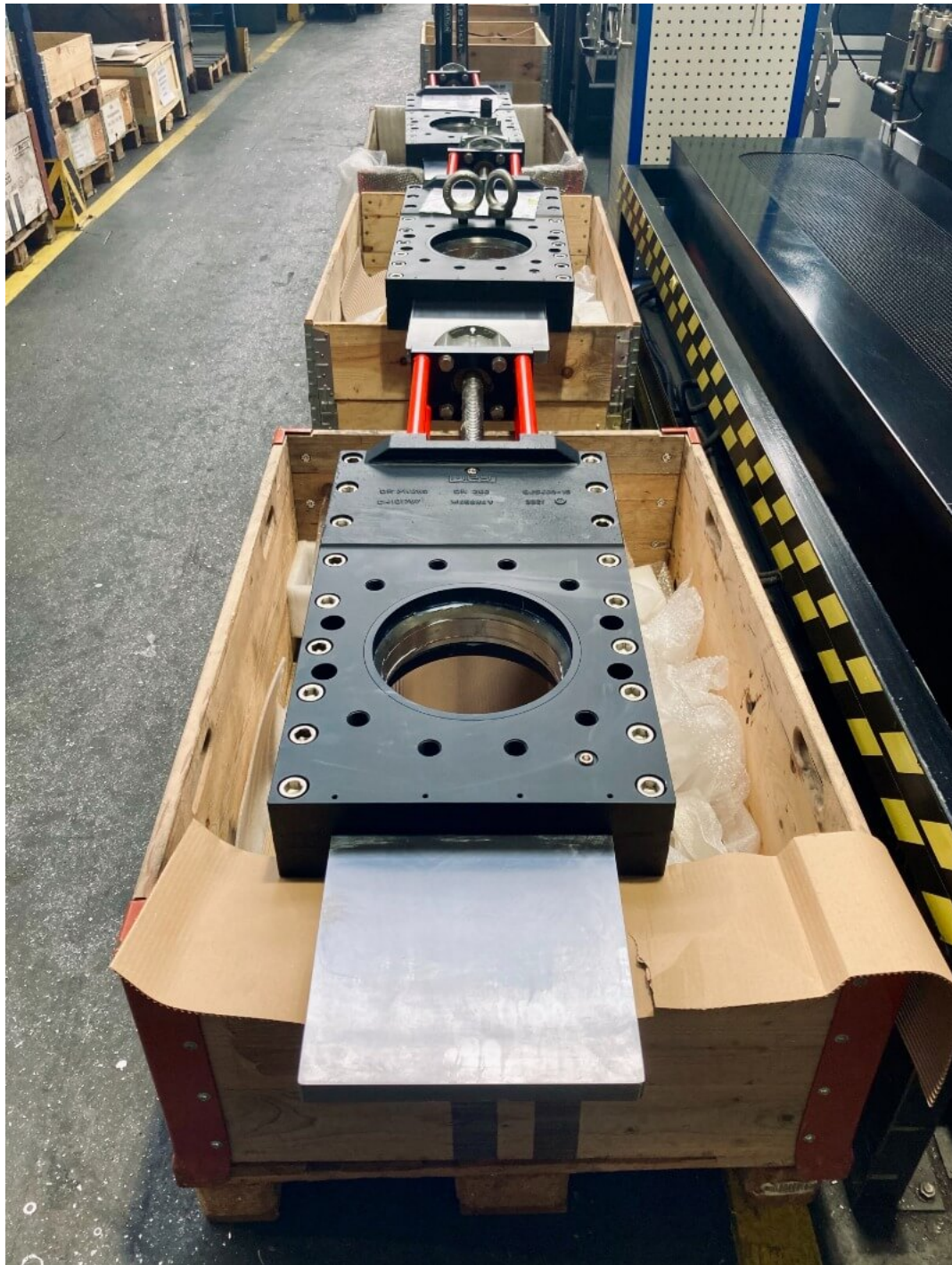
Wey DP made of hardened steel in our production site in Switzerland.
