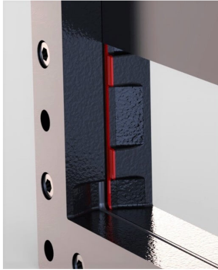
The gate is mechanically guided over the full stroke. Solids are flushed out through the recesses during closing.
