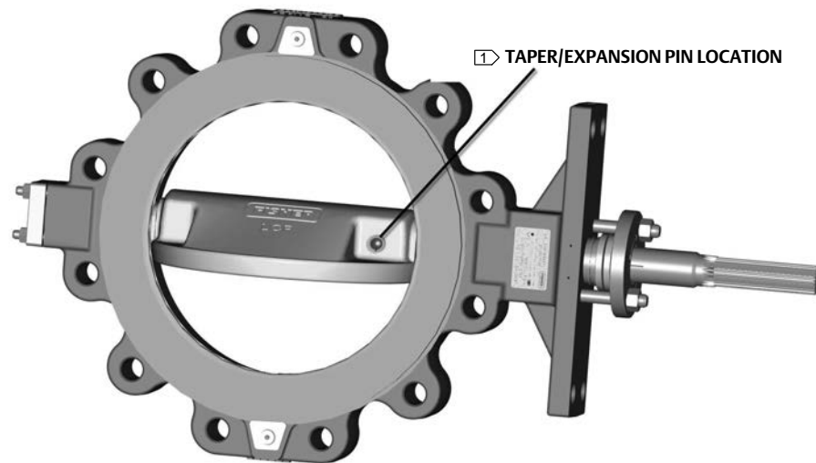
Figure 7. Taper / Expansion Pin Installation
