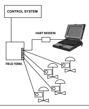
DVC7K digital valve controllers are loop-powered instruments that provide a control valve position proportional to an input signal from the control room. The following describes a double-acting digital valve controller mounted on a piston actuator.
