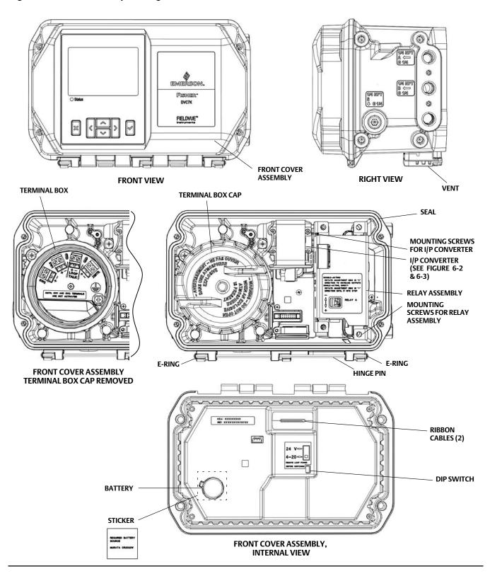
Figure 7-2. DVC7K Assembly Drawings (continued)
