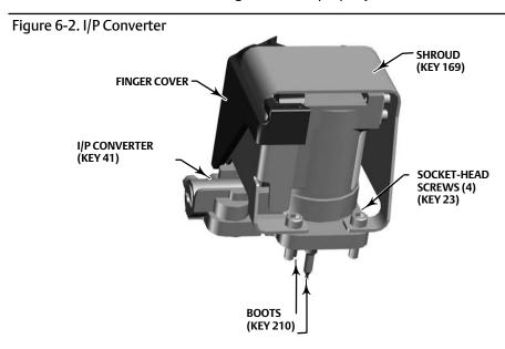
3. Install the I/P converter straight into the module base, taking care that the two electrical leads feed into the guides in the Sensor Assembly.
