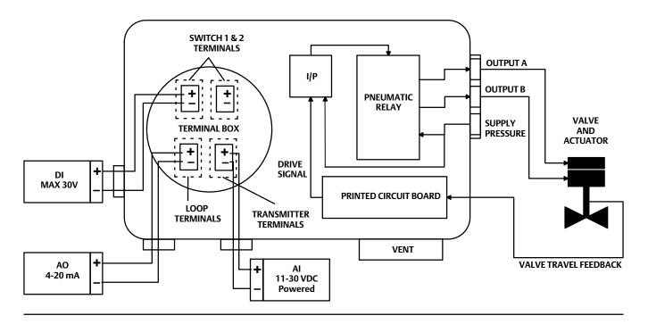
Figure A-5. FIELDVUE DVC7K Digital Valve Controller Assembly
