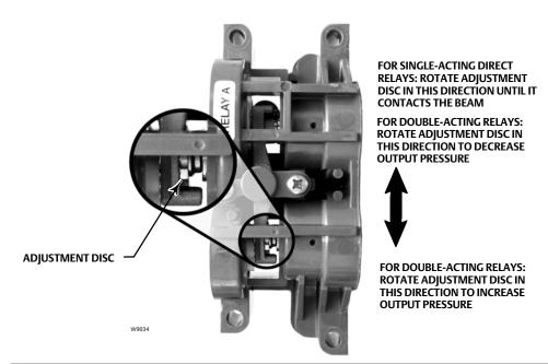
Relay A may also be adjusted for use in single-acting-direct applications. Rotate the adjustment disc as shown in figure 4-1 for single-acting direct operation.
