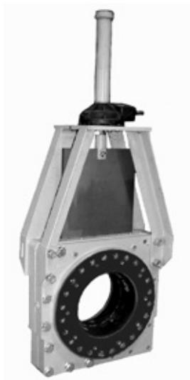
This instruction manual provides installation, operation and maintenance recommendations for both the Clarkson KGF and Clarkson KGF-HP slurry knife gate valves. The standard KGF is a 300 psi CWP valve with optional pressure ratings up to 450 psi cwp and the KGF-HP is rated to Class 300 (740 psi CWP). Both products are very similar, however, the KGF-HP has a higher pressure rating and critical parts are not interchangeable. The KGF and KGF-HP are identified by the valve tag.
