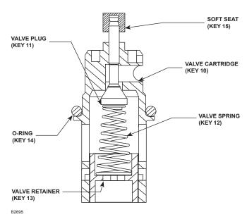
Figure 2. Valve Cartridge Assembly
