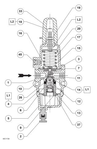
Figure 3. Types 67CFS and 67CFSR Assembly
