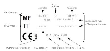
The information on the type plate may vary, depending on the valve model. The traceability of each valve is ensured by the combination of year of manufacture and production number.
