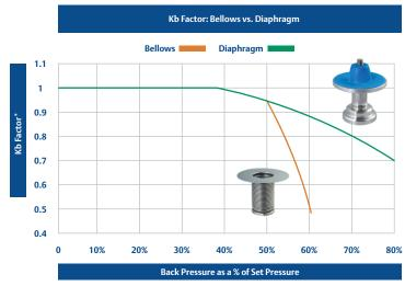
\*Kb = Capacity correction factor due to back pressure
