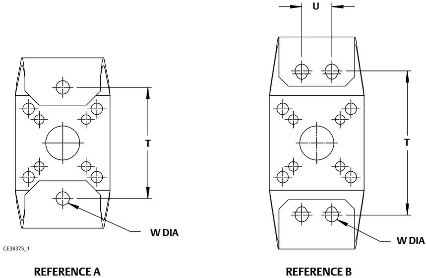
Figure 6. NAMUR Instrument Mounting Dimensions (also see tables 10 and 11)
