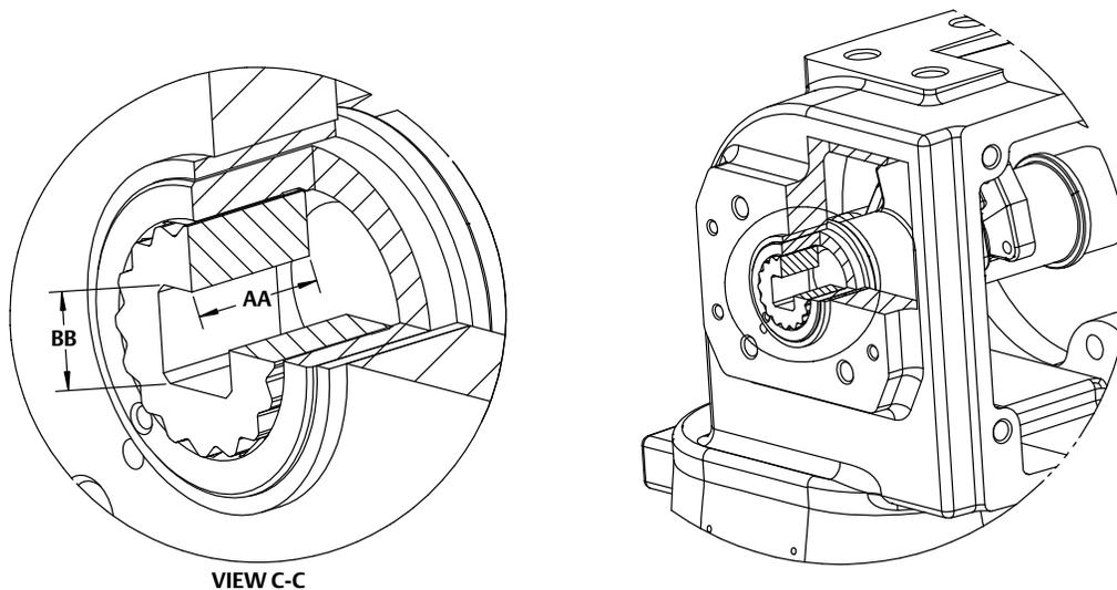
Figure 8. Fisher 2052 Actuator Mounting Styles (also see table 13)
