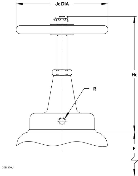
Figure 5. Mounting Yokes Dimensions (also see table 7)
