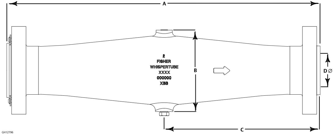
Figure 4. Fisher WhisperTube NPS 4 and NPS 6 Envelope Dimensions
