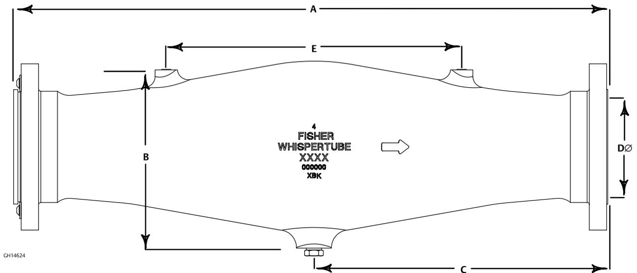
Figure 5. Fisher WhisperTube NPS 8 through 12 Envelope Dimensions
