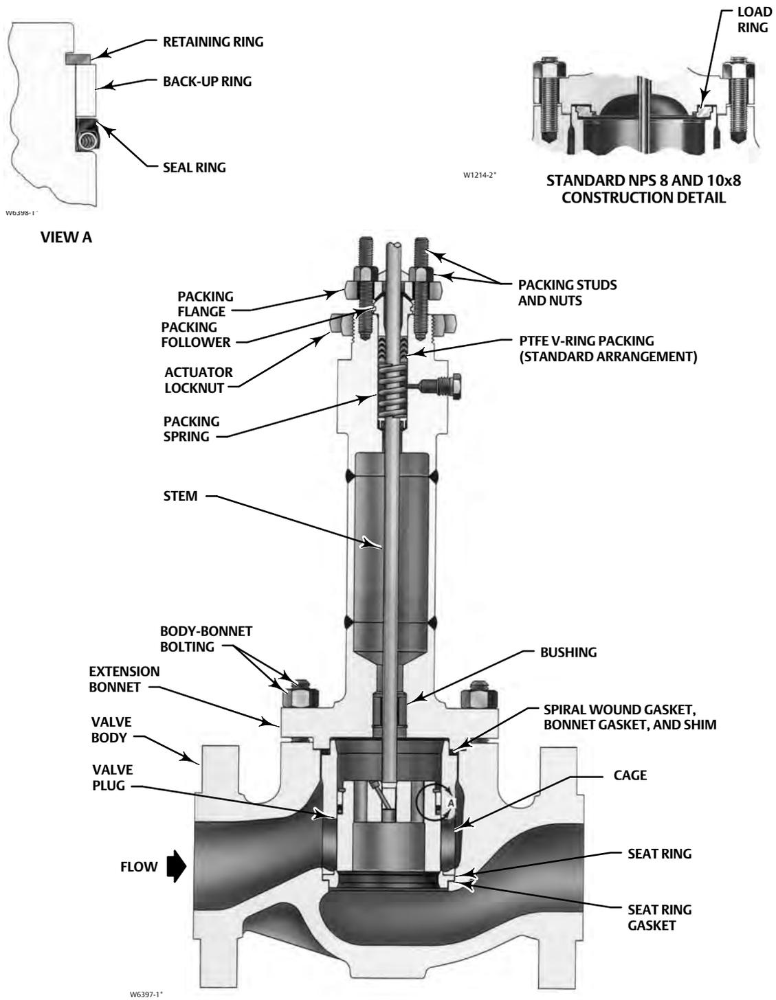
Figure 2. Fisher EZ-C Valve Assembly Detail
