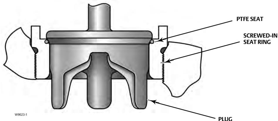
Figure 6. Fisher GX Control Valve with Port-Guided Plug (DN 40 to 150 and NPS 1-1/2 to 6, Port Sizes of 36 - 136mm)
