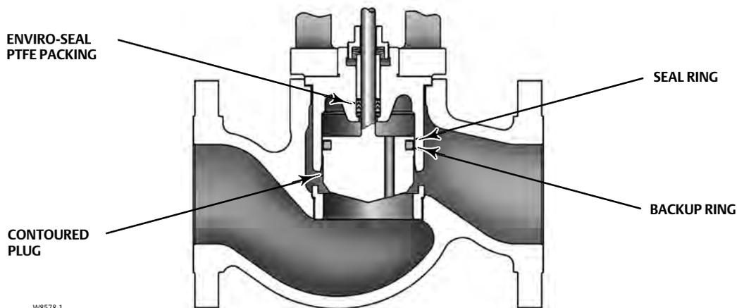
Figure 8. Fisher GX Control Valve Assembly with Stem-Guided Contoured Plug (Size DN 25 and NPS 1)
