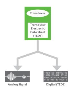
Plug-and-Play Sensors utilize embedded memory chips to recognize and automatically set the sensor range and sensitivity, reducing the need for user input.
