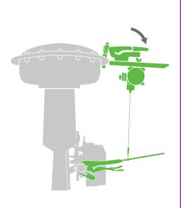
**Quick Connect Fixtures** allow for faster hookup to the valve by using one motion to attach travel transducers that utilize plugand-play technology.
