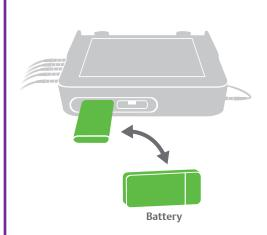
Hot Swappable Batteries can be changed mid-test, eliminating the need for re-testing.
