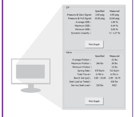
Automated Test Criteria provide a way to define acceptable ranges for critical test variables for added test efficiency, letting you know if a valve falls within the range for a particular parameter.
